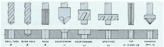
CAD software has a specific Hole tool that can be very handy. Specify diameters and threading based on ANSI and ISO standards (e.g., ANSI #10-32 bolt or ISO M5-0.8). Additionally, a table of holes can be generated Duke BMF on mechanical drawinas.
