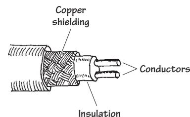
This cable consists of two solid wires insulated from one another by a plastic insulator. Like unbalanced coaxial cable, it too has a copper shielding to reduce noise pickup. Unlike unbalanced coaxial cable, the shielding does not act as one of the conductive paths; it only acts as a shield against external magnetic interference.
