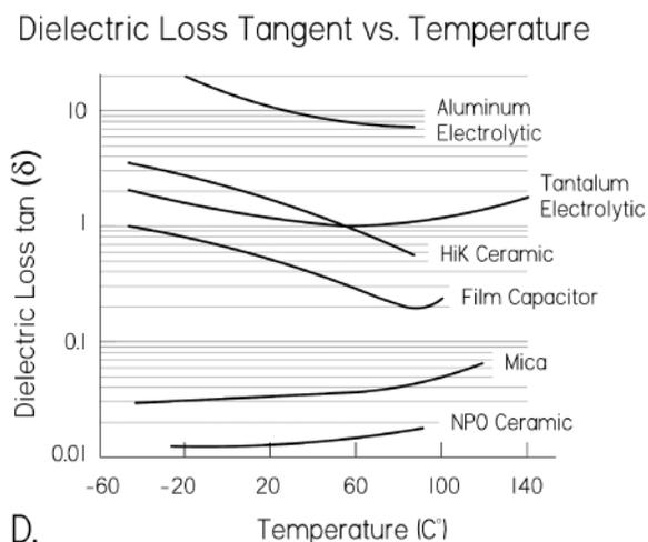
Graph D: Shows the dielectric loss tangent as a function of temperature for various capacitors.
