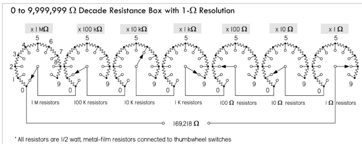
FIGURE 7.67 Resistor decade box made using thumbwheel switches.
