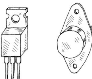
These transistors are used in high-power amplifiers and power supplies. The collector is connected to a metal base that acts as a heat sink. Typical power ratings range from around 10 to 300 W, with frequency ratings from about 1 to 100 MHz. Maximum  $I_C$  values range between 1 to 100 A. They come in *npn*, *pnp*, and Darlington (*npn* or *pnp*) forms.
