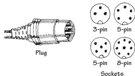
These connectors are used with multiple conductor wires. They are often used for interconnecting audio and computer accessories.
