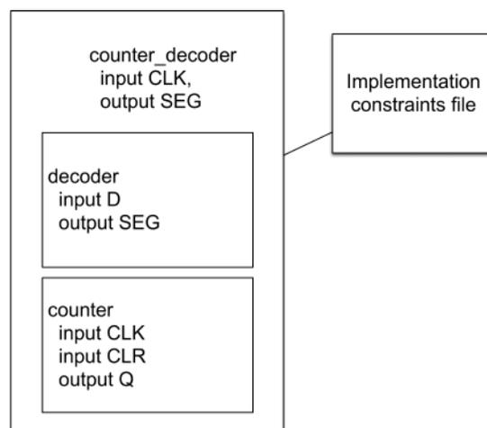
FIGURE 14.28 Counter/decoder modules.
