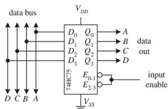
Here a 4-bit data register is created by connecting the enables together to form a single enable input. Data on bus appears at the outputs when the enable input is HIGH. When enable goes LOW, the data that was present on the bus is latched (stored) until latch input goes HIGH.
