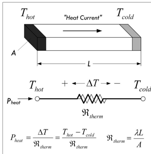
When one end of a block of material is placed at a hot temperature, heat will be conducted through the material to the colder end. The rate of heat transfer, or power due to heating, depends on the thermal resistance of the material, which in turn is dependent on the geometry of the material and the material's thermal resistivity. A weird-looking resistor-like symbol is used here to represent the thermal resistance. Table 2.4 shows the thermal resistivities of various materials.
