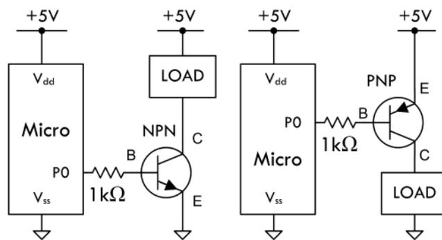
A bipolar transistor can be used to switch on and off loads. In the circuit to the left, when PO is set HIGH, the NPN transistor is turned on—a low resistance is now present between C and E. In the circuit to the right, when PO is set LOW, the PNP transistor is turned on. Microcontroller I/O current levels are usually large enough to provide enough base current for a bipolar transistor. Select a bipolar transistor with the appropriate current/voltage ratings for your load.
