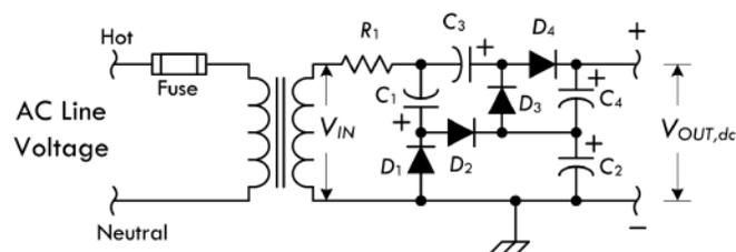
**Voltage quadrupler:** Works in a similar manner as the previous one. In both these circuits, the output voltage will approach an exact multiple of the peak ac voltage when the output current drain is low and the capacitance values high.
