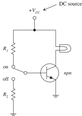
Here, an *npn* transistor is used to control current flow through a light bulb. When the switch is thrown to the on position, the transistor is properly biased, and the collector-to-emitter channel opens, allowing current to flow from  $V_{CC}$  through the light bulb and into ground. The amount of current entering the base is determined by
