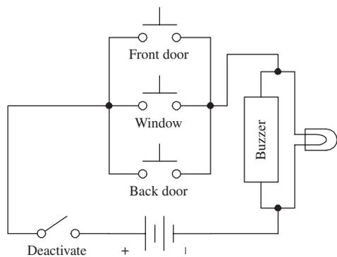
Here’s a simple home security alarm that’s triggered into action (buzzer and light go on) when one of the normally open switches is closed. Magnetic reed switches work particularly well in such applications.
