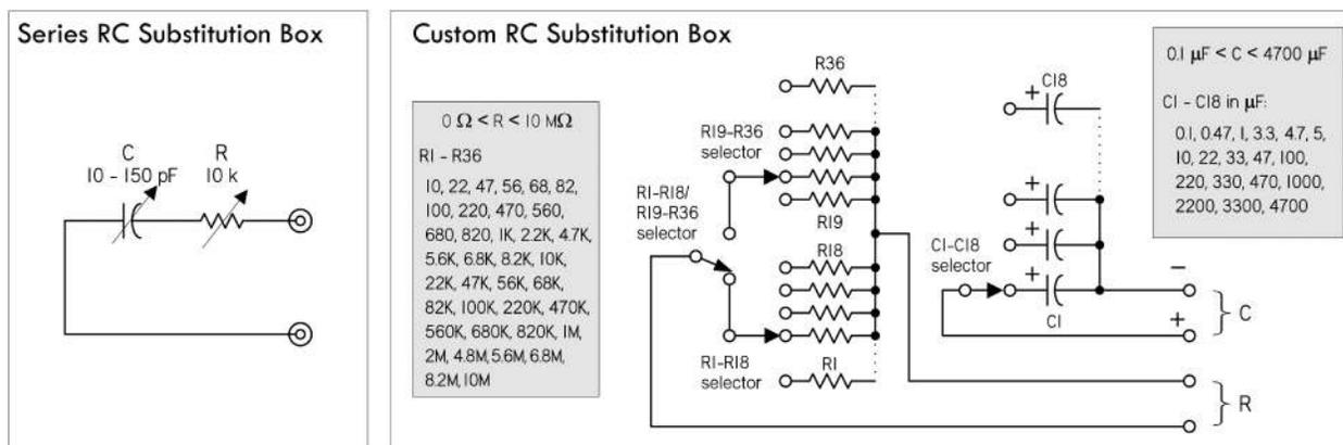
FIGURE 7.68 *Left:* A Series RC substitution box that can be constructed using plastic-film-dielectric tuning capacitor of 10 to 150 pF (or whatever is suitable) and a 10-k $\Omega$ , one-turn potentiometer. *Right:* Custom RC substitution box that can be switched to various modes: resistance-only, capacitance-only, RC-series, and RC-parallel.
