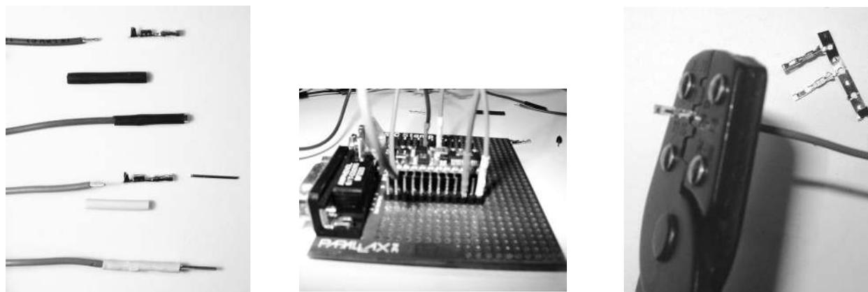
FIGURE 7.75 Making your own stranded-wire, square header jumpers, using hookup wire, female 0.156-in. crimp sockets (solder a 0.100-in. male header pin into the socket for a male jumper), and  $\frac{1}{16}$ - to  $\frac{1}{8}$ -in. shrink tubing. A crimping tool is needed to fasten sockets to wire, although you might get away with using needle-nose pliers and a bit of finesse.
