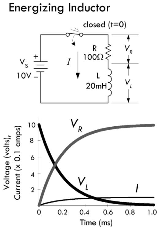
Current and voltage equations for RL energizing circuit:
