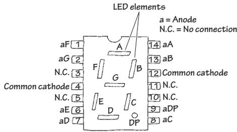
These are used for displaying numbers and other characters. In the LED display shown here, seven individual LEDs are used to make up the display. When a voltage is applied across one of the LEDs, a portion of the 8 lights up. Unlike liquid-crystal displays, LED displays tend to be more rugged, but they also consume more power.
