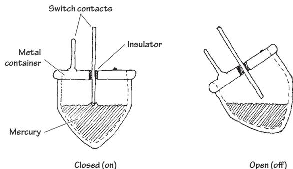
This type of switch is used as a level-sensing switch. In a normally closed mercury tilt-over switch, the switch is “on” when oriented vertically (the liquid mercury will make contact with both switch contacts). However, when the switch is tilted, the mercury will be displaced, hence breaking the conductive path.
