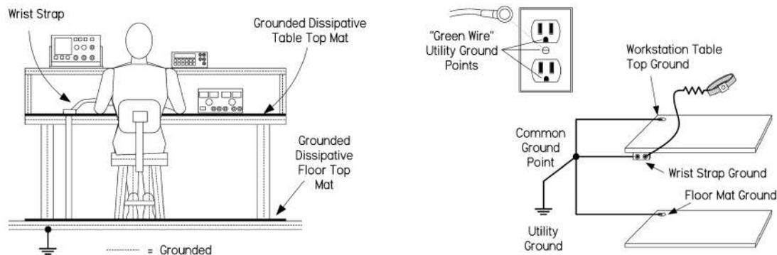
**FIGURE 7.52** A workstation that has been set up to minimize ESD by using grounded dissipative mats and a wrist strap. For reliable grounding, use separate grounding wires for each mat and wrist strap, running them directly to a common ground point.
