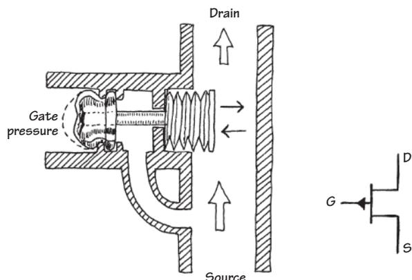
The *p*-channel water JFET is similar to the *n*-channel water JFET, except that all currents and pressures are reversed. The *p*-channel JFET is fully on until a positive pressure, relative to the source, is applied to the gate tube. The positive pressure forces the accordion across the drain-source channel, hence reducing the current flow.
