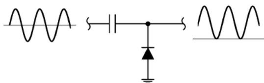
The diode voltage clamp provides dc restoration of a signal that has been ac-coupled (capacitively coupled). This is important for circuits whose inputs look like diodes (e.g., a transistor with grounded emitter); otherwise, an ac-couple signal would fade away.
