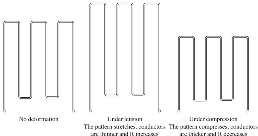
**FIGURE 6.23 Strain gauge.**
