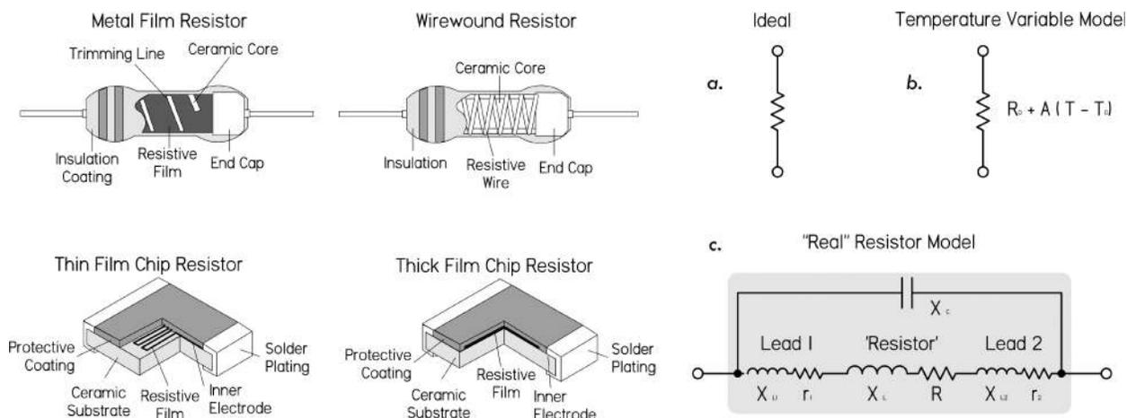
**FIGURE 3.53** Some examples of real resistor construction, as well as various resistor models that are used to aid in predicting how a real resistor will behave. Model (a) represents an ideal resistor, while model (b) represents a temperature variable model for noninductive resistors. Model (c) takes into consideration the inherent inductive and capacitive elements within a resistor's construction. For UHF and microwave designs, model (c) could be used with  $L$  representing lead inductances.
