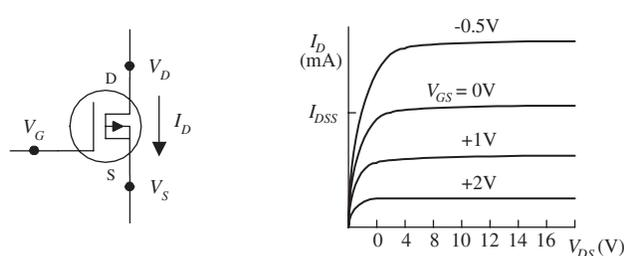
**TRANSCONDUCTANCE ( $g_m$ )** Represents the rate of change in the drain current with
