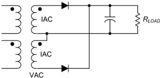
(d) *Full-wave center tap*: While more efficient than the half-wave rectifier circuit, the full wave does not make full use of secondaries, but is good for high-current, low-voltage applications, as there is only one diode drop per positive half cycle.
