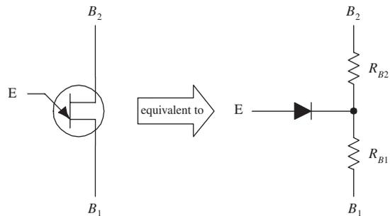
Figure 4.107 shows a typical  $V_E$  versus  $I_E$  graph of an UJT, as well as a UJT equivalent circuit. In terms of the UJT theory, if  $B_1$  is grounded, a voltage applied to the emitter will have no effect (does not increase conductance from one base to another) until it exceeds a critical voltage, known as the *triggering voltage*. The triggering voltage is given by the following expression:
