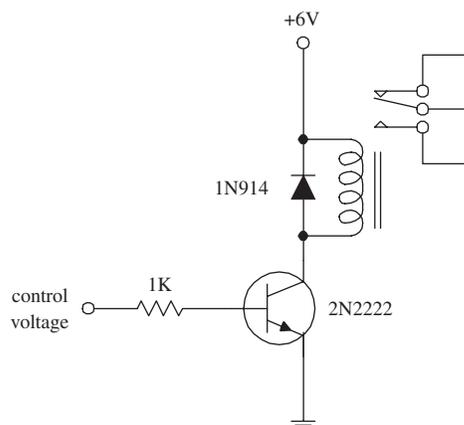
Here, an *np*n transistor is used to control a relay. When the transistor’s base receives a control voltage/current, the transistor will turn on, allowing current to flow through the relay coil and causing the relay to switch states. The diode is used to eliminate voltage spikes created by the relay’s coil. The relay must be chosen according to the proper voltage rating, etc.
