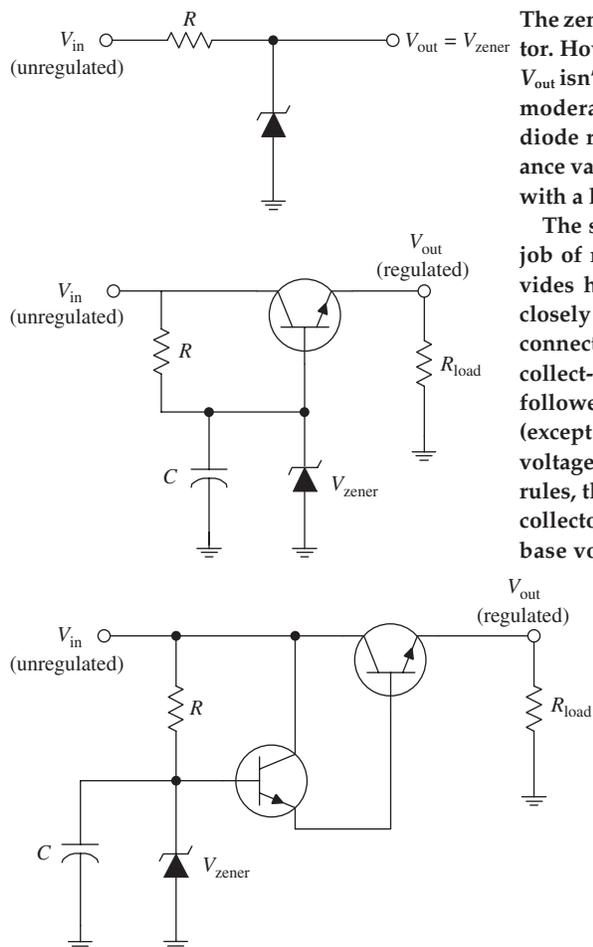
The zener diode circuit here can be used to make a simple voltage regulator. However, in many applications, the simple regulator has problems;  $V_{out}$  isn’t adjustable to a precise value, and the zener diode provides only moderate protection against ripple voltages. Also, the simple zener diode regulator does not work particularly well when the load impedance varies. Accommodating large load variations requires a zener diode with a large power rating—which can be costly.
