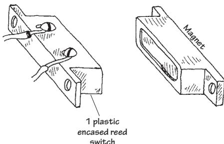
A reed switch consists of two closely spaced leaflike contacts that are enclosed in an air-tight container. When a magnetic field is brought nearby, the two contacts will come together (if it is a normally open reed switch) or will push apart (if it is a normally closed reed switch).
