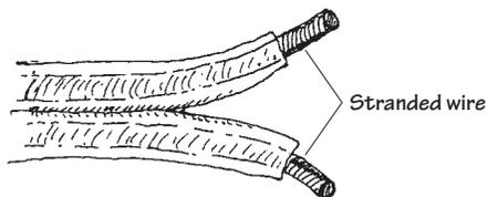
This wire is stranded to increase surface area for current flow. It has a high copper content for better conduction.
