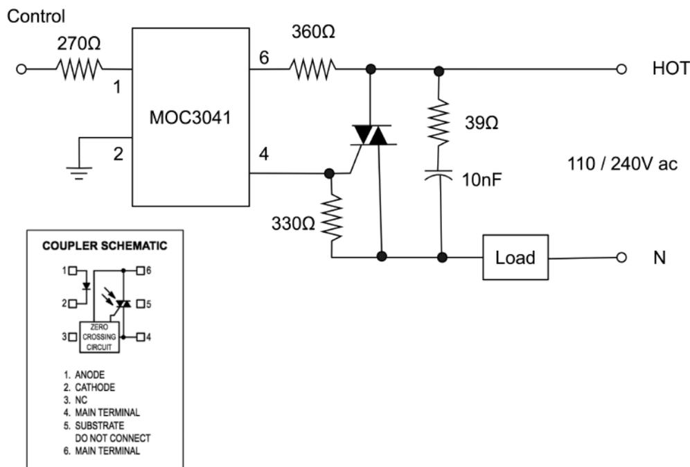
Optoisolated triacs like the MOC3041 have zero-crossing detection built in so that they turn on only at the zero-crossing point, minimizing current surges. This device can be used to control a regular triac to switch 110 V ac.
