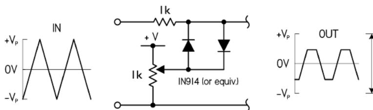
The adjustable attenuator is similar to the last circuit, but the additional opposing diode allows for clipping on both positive and negative swings. You can use separate potentiometers if you want separate positive and negative clipping level control. +V should be a volt or so higher than the peak input voltage.
