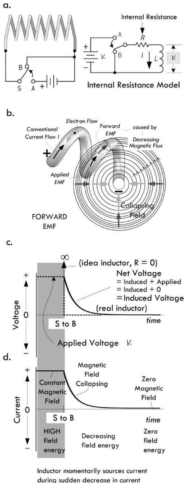
When an inductor is being deenergized, we say that the magnetic field energy of the inductor is “transformed” back into electrical energy. Again, only during times of change, which in our case involves a decreasing current flow, do we notice effects of induction.
