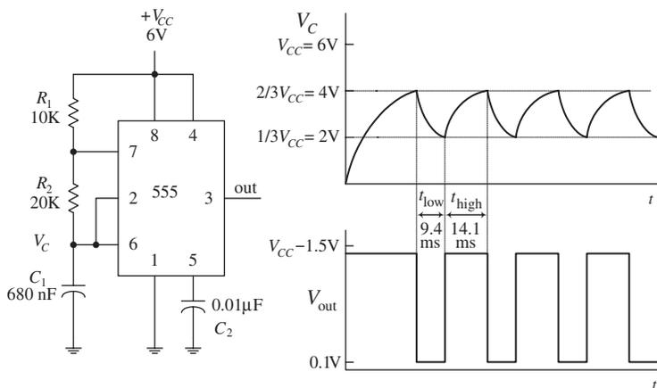
$$t_{\text{low}} = 0.693(20\text{K})(680\text{nF}) = 9.6\text{ms}$$
