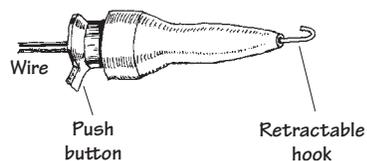
These connectors are used as test probes. The spring-loaded hook opens and closes with the push of a button. The hook can be clamped onto wires and component leads.
