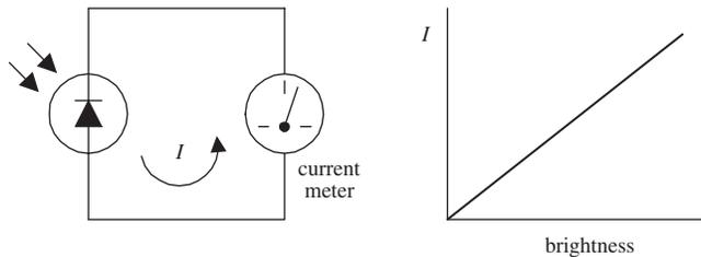
Here, a photodiode acts to convert light energy directly into electric current that can be measured with a meter. The input intensity of light (brightness) and the output current are nearly linear.
