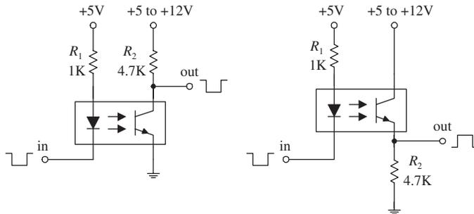
Here, a diode/phototransistor optoisolator is used to provide electrical isolation between the source circuit and the sensor circuit, as well as providing a dc level shift in the output. In the leftmost circuit, the output is noninverted, while the output in the rightmost circuit is inverted.
