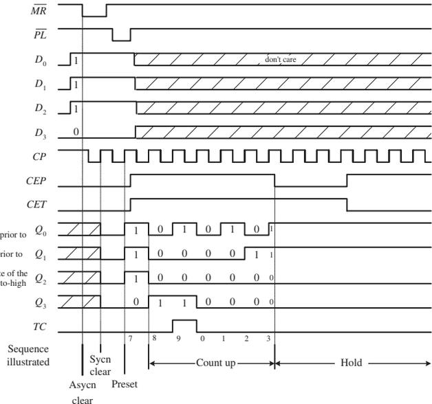
Synchronous multistage counter using the 74163
