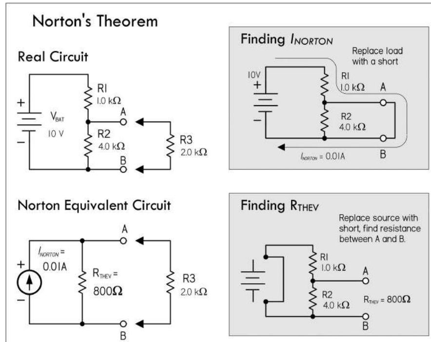
FIGURE 2.73 To find  $I_{\text{NORTON}}$ , first remove load  $R_3$  and replace it with a short. Using Ohm's law, and noticing that no current will ideally flow through  $R_2$  since it's shorted, you find the short-circuit current, or Norton current, to be:
