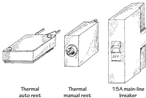
These come in both rocker and push-button forms. Some have manual resets, while others have thermally actuated resets (they reset themselves as they cool down). Main-line circuit breakers are rated at 15 to 20 A. Smaller circuit breakers may be rated as low as 1 A.
