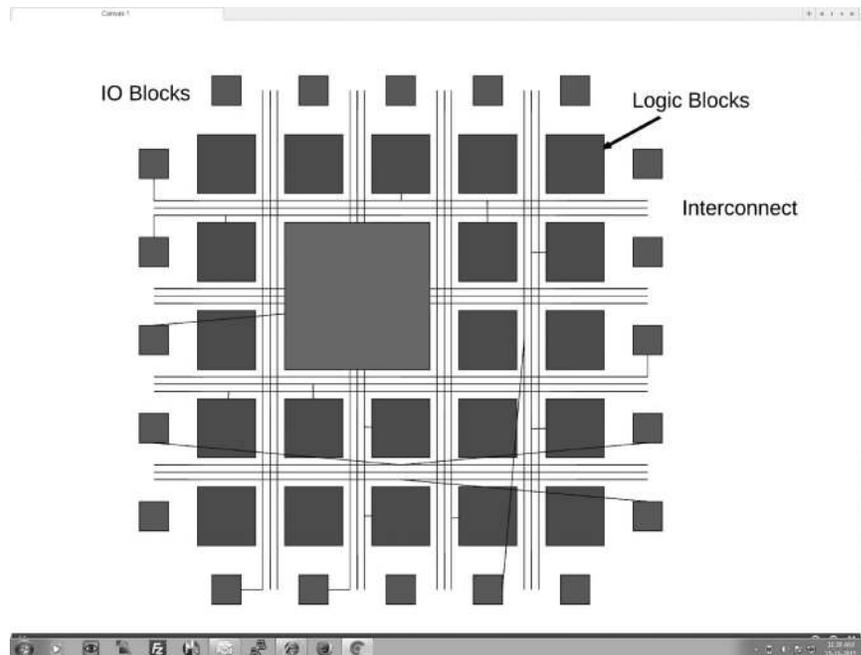
FIGURE 14.3 The logical structure of an FPGA.
