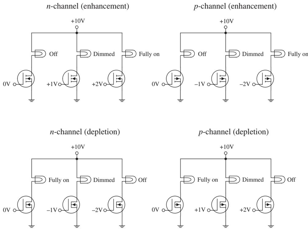
The circuits shown here demonstrate how MOSFETs can be used to control current flow through a light bulb. The desired dimming effects produced by the gate voltages may vary depending on the specific MOSFET you are working with.
