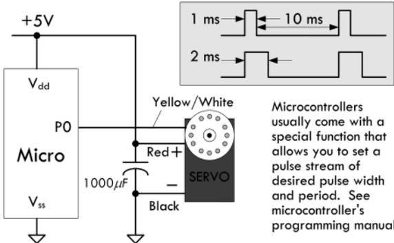
Microcontrollers usually come with a special function that allows you to set a pulse stream of desired pulse width and period. See microcontroller's programming manual.
