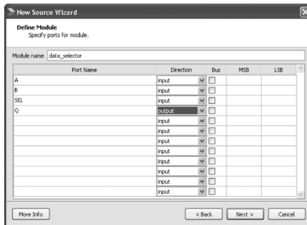
FIGURE 14.25 Defining inputs and outputs for the new Verilog source.
