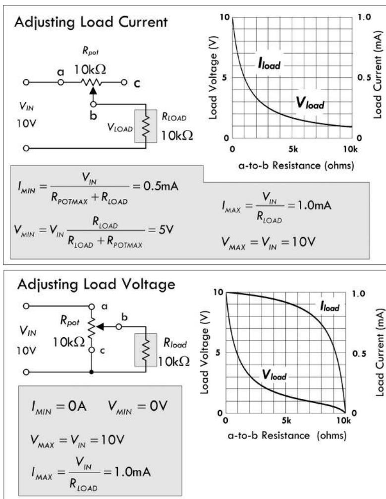
*Adjusting load current:* Here, a pot's variable resistance element (a-to-b) is in series with a load. Adjusting manual control of the pot alters the current to the load. The current as a function of pot resistance is:
