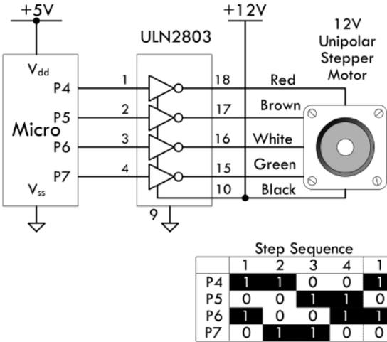
Here a 12V unipolar stepper motor is controlled using a TTL open collector driver IC connected to microcontroller. The step sequence for rotating motor is shown to the left. There are many new stepper motor drivers circuits out there that have many bells and whistles. Your best bet is to check the Internet to see what new technology exists and to study various example codes used to drive the stepper motors.
