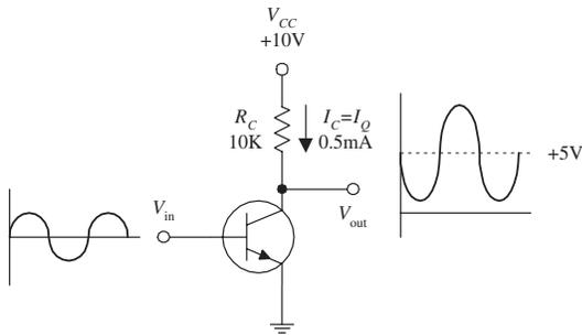
The transistor configuration here is referred to as the *common-emitter configuration*. Unlike the emitter follower, the common emitter has voltage gain. To figure out how this circuit works, first set  $V_C = \frac{1}{2}V_{CC}$  to allow for maximum swing without clipping. Like the emitter follower, again pick a quiescent current  $I_Q$  to start with. To set  $V_C = \frac{1}{2}V_{CC}$  with a desired  $I_Q$ , use  $R_C$ , which is found by Ohm's law:
