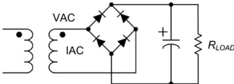
(b) *Full-wave bridge*: Most efficient use of transformer's secondary winding. Best for high-voltage outputs.
