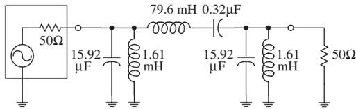
The important part comes now. Each circuit branch of the low-pass filter must be resonated to  $f_0$  by adding a series capacitor to each inductor and a parallel inductor to each capacitor. The LC resonant equation is used to determine the additional component values:
