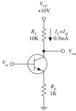
For example, if  $V_{CC}$  is 10 V and  $I_Q$  is 0.5 mA,  $R_C$  is then 10 k. The gain of this circuit is found by realizing that  $\Delta V_E = \Delta V_B$  (where  $\Delta$  represents a small fluctuation). The emitter current is found using Ohm's law:
