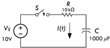
$$I(t) = \begin{cases} 0 & t < 0 \text{ (before S closed)} \\ V_S / R & t = 0 \text{ (S just closed)} \\ (V_S / R)e^{-t/RC} & t > 0 \text{ (after S closed)} \\ 0 & t \rightarrow \infty \text{ (steady state)} \end{cases}$$
