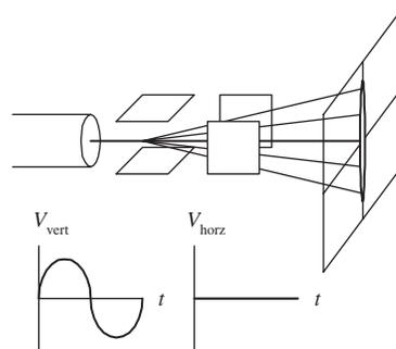
When a sinusoidal voltage is applied to the vertical plates, while no voltage is applied to the horizontal plates, a vertical line is traced on the y axis.
