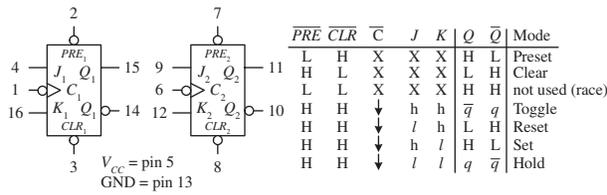
74109 dual JK positive edge-triggered flip-flop with Preset and Clear
