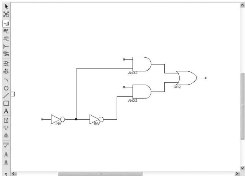
FIGURE 14.13 Connecting the symbols with wires.
