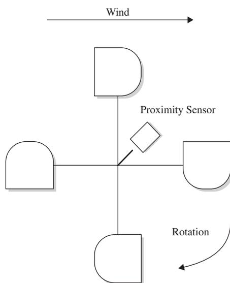
**FIGURE 6.22** A cup anemometer.
