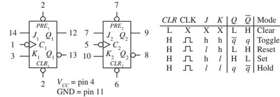
74114 dual pulse-triggered JK flip-flop with common Clock
