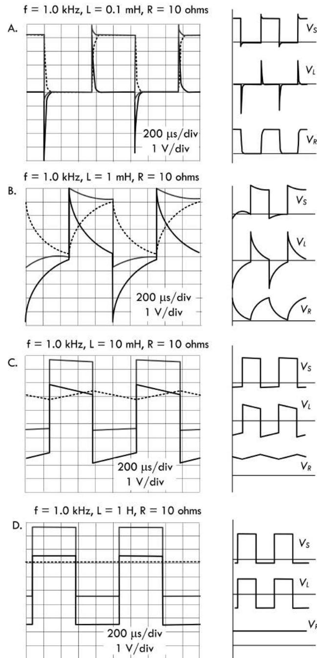
Inductance, be it intended or not, can have a major influence on signals. For example, the output signals across the inductor and resistor in the RL circuit to the left become increasingly distorted as the inductance increases. With a constant 1.0-kHz, 0–5-V squarewave source, and fixed 10-Ω resistance, we increase the inductance and note the changes in the waveforms. First we note that the period of the squarewave is:
