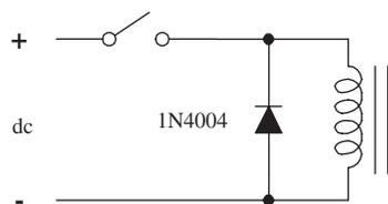
Placing a diode in reverse bias across a relay's coil eliminates voltage spikes by going into conduction before a large voltage can form across the coil. The diode must have a peak current capability able to handle currents equivalent to the maximum current that would have been flowing through the coil before the current supply was interrupted. A good general-purpose diode that works well for just such applications is the 1N4004 diode.
