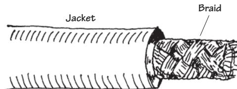
A braided wire is made up of a number of individual strands of wire braided together. Like stranded wires, these wires are better conductors than solid-core wires, and they will not break easily when flexed. Braided wires are frequently used as an electromagnetic shield in noise-reduction cables and also may act as a wire conductor within the cable (e.g., coaxial cable).
