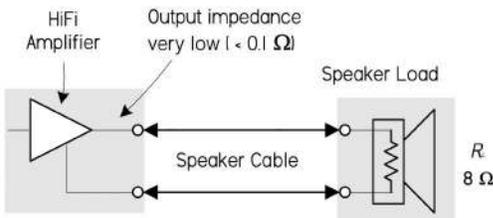
Virtually all audio power from amplifier is transferred into speaker.
