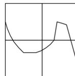
The scope no longer uses the x axis as the time axis, but uses signal voltage from another external source.
