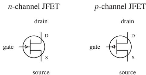
JFETs come in either *n-channel* or *p-channel* configurations. With an *n-channel* JFET, a negative voltage applied to its gate (relative to its source lead) reduces current flow from its drain to source lead. (It operates with  $V_D > V_S$ .) With a *p-channel* JFET, a positive voltage applied to its gate reduces current flow from its source to drain lead. (It operates with  $V_S > V_D$ .) The symbols for both types of JFETs are shown at the left.
