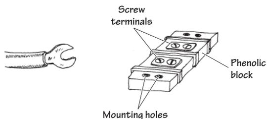
This is a simple connector that uses a screw to fasten a metal spade to a terminal. A barrier strip often acts as the receiver of the spade lugs.
