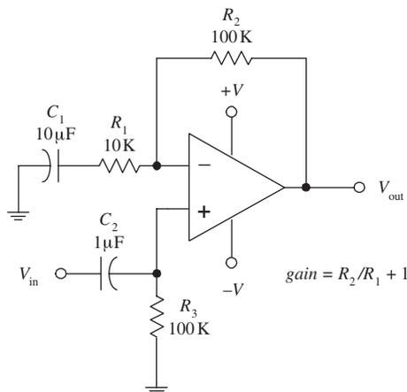
Noninverting amplifier (single power supply)
