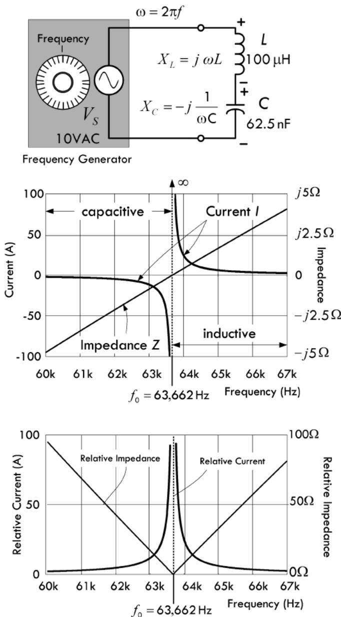
**Example:** To get an idea of how the LC series circuit works, we find the equivalent impedance of the circuit—taking  $L$  and  $C$  in series. Unlike the previous examples, the frequency is unknown, so it must be left as a variable:
