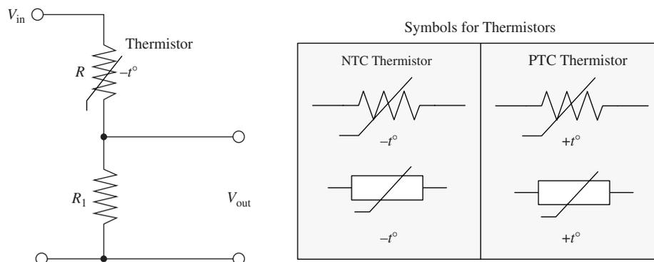
FIGURE 6.6 Using a thermistor as a thermometer.
