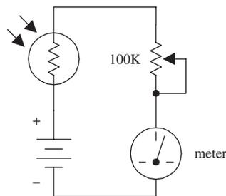
Here, a photoresistor acts as the light-sensing element in a simple light meter. When dark, the photoresistor is very resistive, and little current flows through the series loop; the meter is at its lowest deflection level. When an increasingly bright light source is shone on the photoresistor, the photoresistor's resistance begins to decrease, and more current begins to flow through the series loop; the meter starts to deflect. The potentiometer is used to adjust the sensitivity of the meter.
