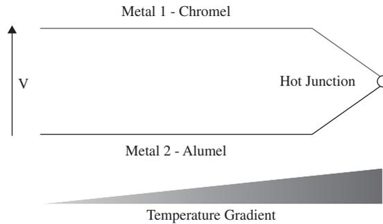
FIGURE 6.7 Thermocouples.
