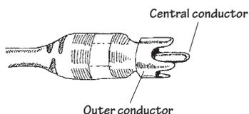
Phono connectors are often referred to as RCA plugs or pin plugs. They are used primarily in audio connections.
