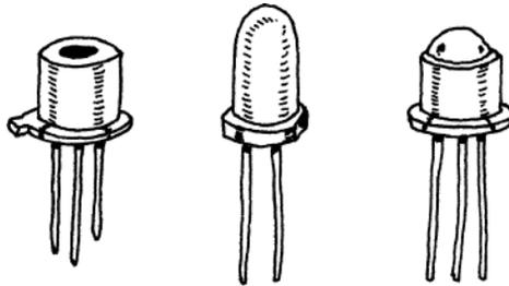
This transistor acts as a light-sensitive bipolar transistor (base is exposed to light). When light comes in contact with the base region, a base current results. Depending on the type of phototransistor, the light may act exclusively as a biasing agent (two-lead phototransistor) or may simply alter an already present base current (three-lead phototransistor). See Chap. 5 for more details.
