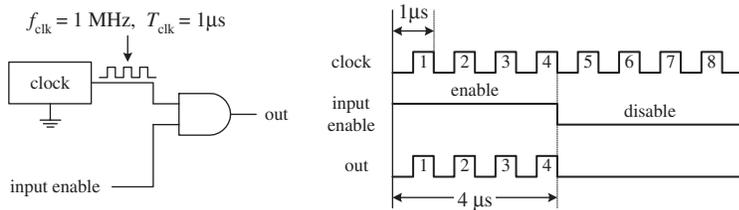
In the upper part of the figure, an AND gate acts as the enable gate. When the input enable lead is made high, the clock signal will pass to the output. In this example, the input enable is held high for 4  $\mu\text{s}$ , allowing 4 clock pulses (where  $T_{\text{clk}} = 1 \mu\text{s}$ ) to pass. When the input enable lead is low, the gate is disabled, and no clock pulses make it through to the output.
