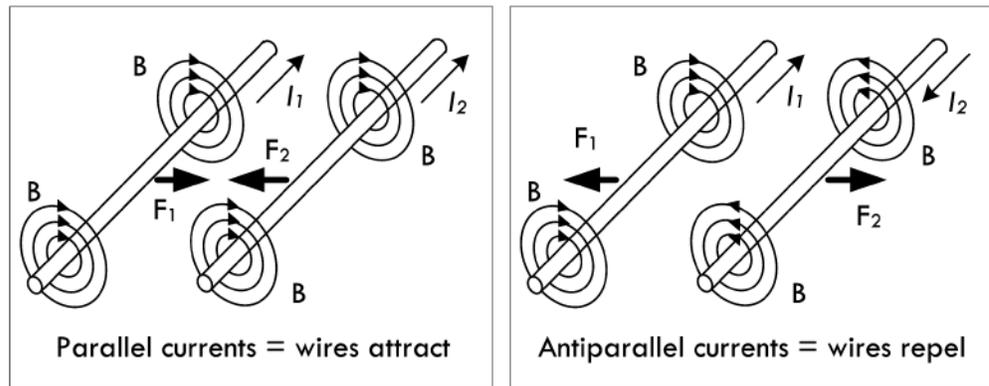
FIGURE 2.114 Forces exerted between two current-carrying wires.
