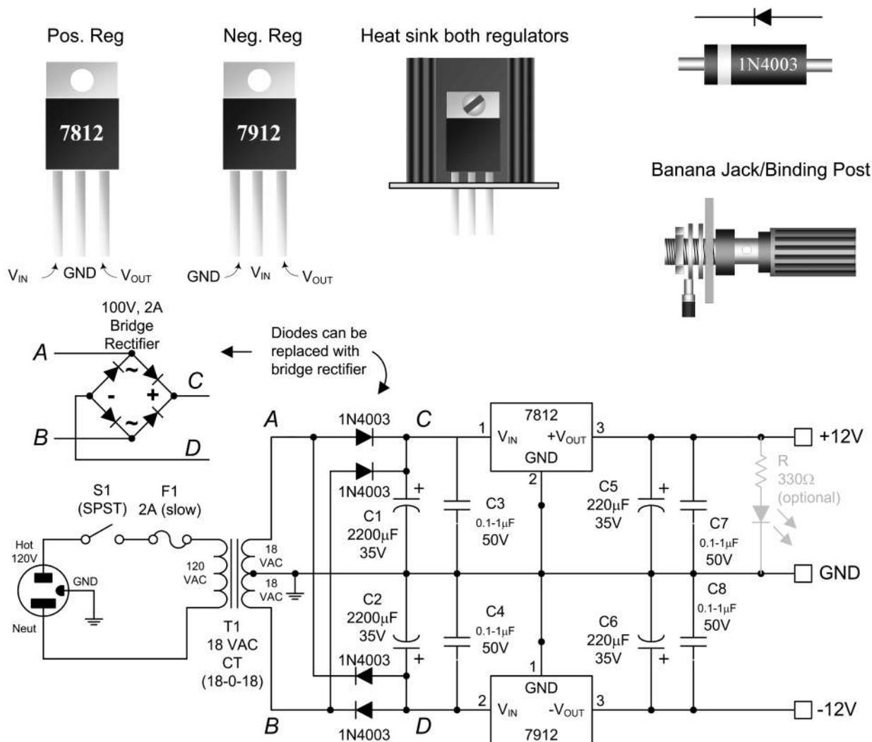
FIGURE 11.10c Here's a fixed  $\pm 12$  V made by using a center-tap 18-VAC transformer, a full-wave rectifier, and 7812 and 7912 regulators. This circuit is particularly useful when powering op amp circuits.
