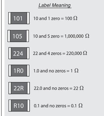
The first two digits represent significant figures; the last digit specifies the multiplier. For values under 100  $\Omega$ , the letter R is substituted for one of the significant digits and represents a decimal point.
