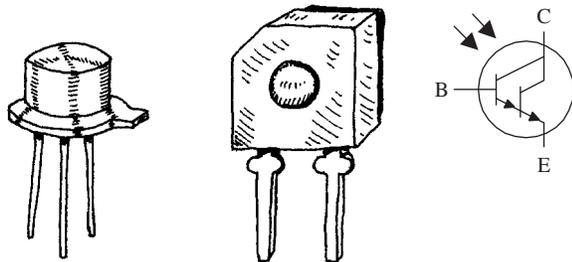
This is similar to a conventional bipolar Darlington transistor but is light-sensitive. Photodarlingtons are much more sensitive to light than ordinary phototransistors, but they tend to have slower response times. These devices may or may not come with a base lead.
