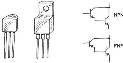
These are two transistors in one. They provide more stability at high current levels. The effective  $h_{FE}$  for the device is much larger than that of a single transistor, hence allowing for a larger current gain. They come in *nnp* (*D-npn*) and *ppp* (*D-pnp*) Darlington packages.
