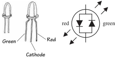
Multicolor LEDs mount a number of LEDs in a single package. The color they produce is a mixture of the colors produced by each LED. The ultimate multicolor LED is an RGB LED that has red, green, and blue LEDs within a single package. This allows any color to be mixed by controlling the brightness of each of the LEDs, with white light being produced if all the LEDs are on with equal intensity. The packages usually have a common anode or common cathode connection.
