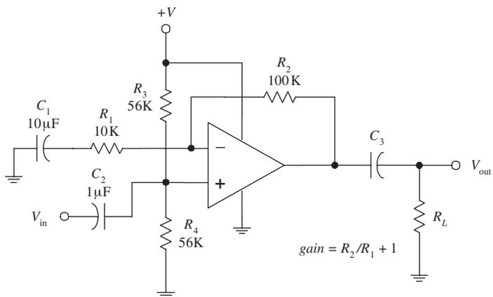
FIGURE 16.7 Components  $R_1$ ,  $C_1$ ,  $R_2$ , and the biasing resistors serve the same function as was seen in the inverting amplifier circuits. The noninverting input offers an exceptionally high input impedance and can be matched to the source impedance more readily by adjusting  $C_2$  and  $R_3$  (dual-supply circuit) or  $R_4$  (single-supply circuit). The input impedance is approximately equal to  $R_3$  (dual-supply circuit) or  $R_4$  (single-supply circuit).
