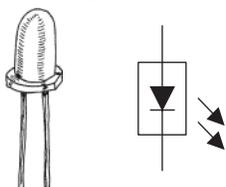
These LEDs contain a miniature integrated circuit within their package that causes the LED to flash from 1 to 6 times each second. They are used primarily as indicator flashers, but may be used as simple oscillators.
