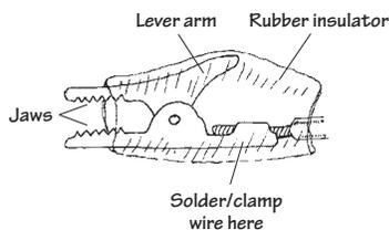
Alligator connectors are used primarily as temporary test leads.
