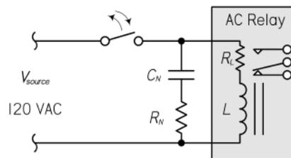
The circuit that is used is dependent on the particular situation. Either circuit may provide enough protection for a given application. For extreme cases, both load and contact protection may be required.
