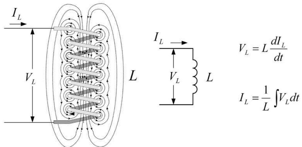
**FIGURE 2.127** The voltage measured across an ideal inductor is the induced voltage, or EMF, symbolized  $V_L$ . When there is a steady-state dc current flow, there is no induced voltage ( $V_L$  is zero) and the inductor resembles a short. As we'll see, the inductor equations can yield surprisingly unrealistic values, if we don't consider internal resistance and capacitance inherently present within a real inductor.
