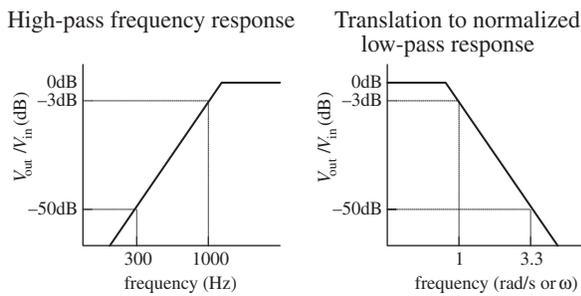
The first step is to convert the high-pass response into a normalized low-pass response, as shown in the figure. The steepness factor for the low-pass equivalent response is given by
