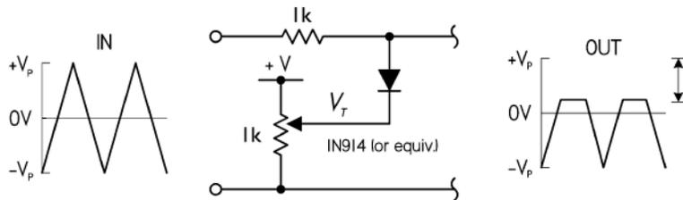
In the adjustable waveform clipper circuit, the maximum output is clipped to a level determined by the resistance of the potentiometer. The idea is to set the negative end of the diode to about 0.6 V lower than the maximum desired output level, to account for the forward voltage drop of the diode. That's what the potentiometer is intended to do. +V should be a volt or so higher than the peak input voltage.
