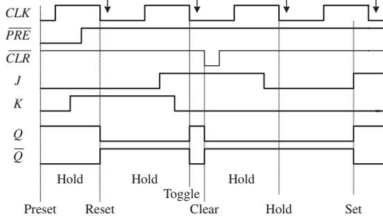
Negative edge-triggered JK flip-flop with Preset and Clear
