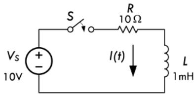
$$I(t) = \begin{cases} 0 & t < 0 \text{ (before S closed)} \\ 0 & t = 0 \text{ (S just closed)} \\ (V_S / R)(1 - e^{-(R/L)t}) & t > 0 \text{ (after S closed)} \\ V_S / R & t \rightarrow \infty \text{ (steady state)} \end{cases}$$
