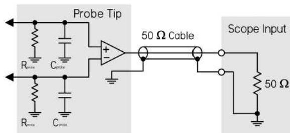
34 MHz). The 10X probe introduces about ten times less capacitance. Bandwidth differences also apply to 100X and 1000X probes.
