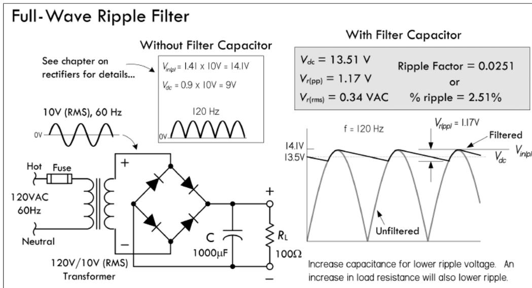
FIGURE 3.73 Here, a 1000- $\mu F$  capacitor supply filter is used to reduce the output ripple voltage. With a 100- $\Omega$  load, the ripple voltage in this circuit is 0.34 VAC, or 1.17 V peak to peak. The ripple factor (rms ripple voltage divided by average dc voltage) is 0.00251. If we replaced the full-wave bridge with a half-wave rectifier, the ripple voltage would be twice as large. See equations in Fig. 3.74 and Problem 7 at the end of this chapter.
