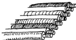
This type of cable is used in applications where many wires are needed. It tends to flex easily. It is designed to handle low-level voltages and often is found in digital systems, such as computers, to transmit parallel bits of information from one digital device to another.
