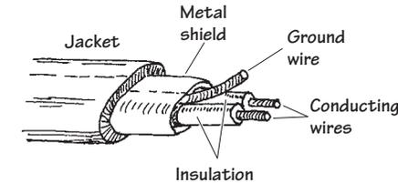
This cable is similar to paired cable, but the inner wires are surrounded by a metal-foil wrapping that's connected to a ground wire. The metal foil is designed to shield the inner wires from external magnetic fields—potential forces that can create noisy signals within the inner wires.
