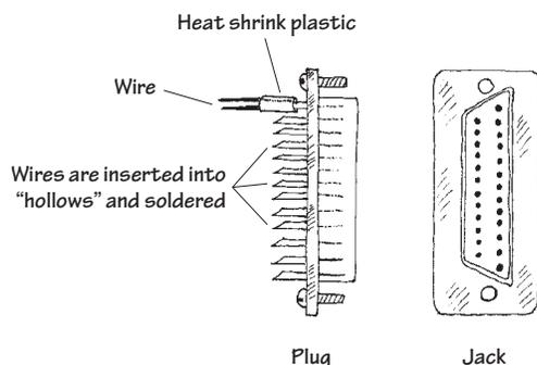
D-connectors are used with ribbon cable. Each connector may have as many as 50 contacts. The connection of each individual wire to each individual plug pin or jack socket is made by sliding the wire in a hollow metal collar at the backside of each connector. The wire is then soldered into place.
