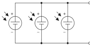
Like batteries, solar cells can be combined in series or parallel configurations. Each solar cell produces an open-circuit voltage from around 0.45 to 0.5 V and may generate as much as 0.1 A in bright light. By adding cells in series, the output voltage becomes the sum of the individual cell voltages. When cells are placed in parallel, the output current increases.
