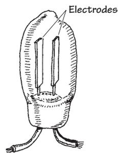
This lamp produces a dim, pale light that results from the ionization of neon gas molecules between two electrodes within the bulb. Types of gas-discharge lamps include neon, xenon flash, and mercury vapor lamps. Gas-discharge lamps have a tendency to suddenly switch on when a particular minimum operating voltage is met. For this reason, they are sometimes used in triggering and voltage-regulation applications. They are also used as indicator lights and for testing home ac power outlets.
