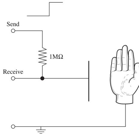
FIGURE 6.15 Capacitive sensing.
