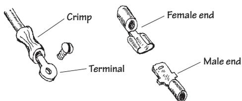
Crimp connectors are color-coded according to the wire size they can accommodate. They are useful as quick, friction-type connections in dc applications where connections are broken repeatedly. A crimping tool is used to fasten the wire to the connector.
