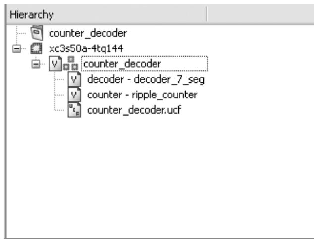
FIGURE 14.29 The Hierarchy View indicating the top-level module.
