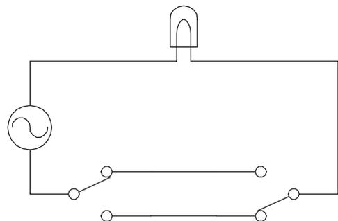
Here’s a switch network that allows an individual to turn a light on or off from either of two locations. This setup is frequently used in household wiring applications.
