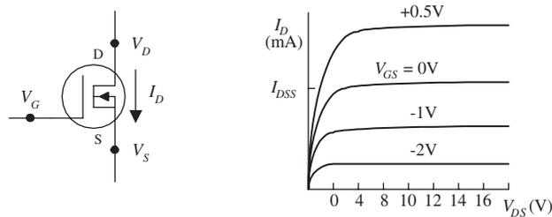
**OHMIC REGION** MOSFET is just beginning to resist. In this region, the MOSFET behaves like a variable resistor.
