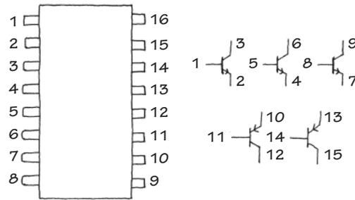
This consists of a number of transistors combined into a single integrated package. For example, the transistor array shown here is made of three *nnp* transistors and two *ppp* transistors.
